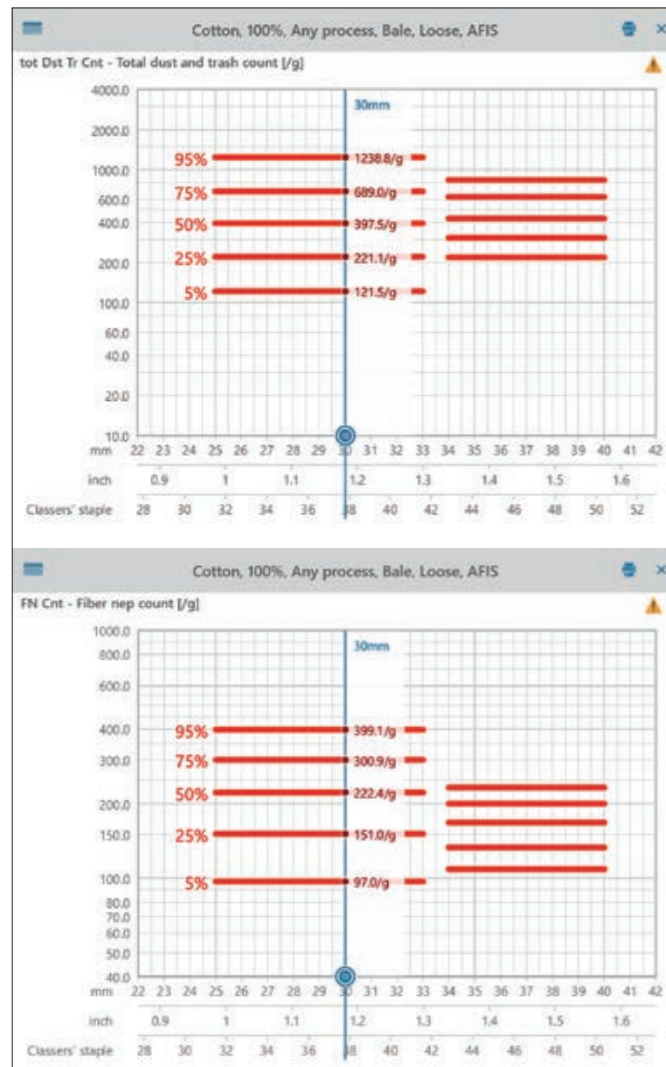
Fig. 24 New graphs for total dust and trash count, as well as fiber nep count
