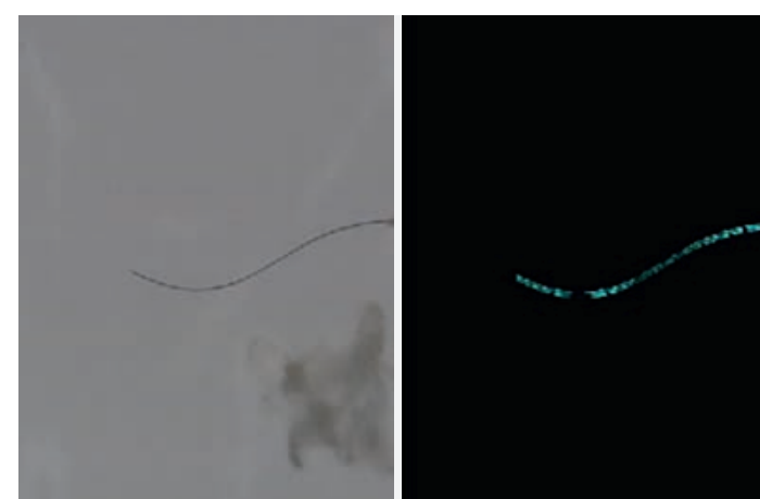
Left: Contaminant (hair) within cotton Right: Contaminant (hair) separated after Quick Teach
