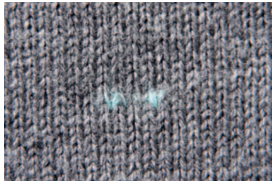
Top: Fabric with a claim from a few thick and thin outlier bobbins
